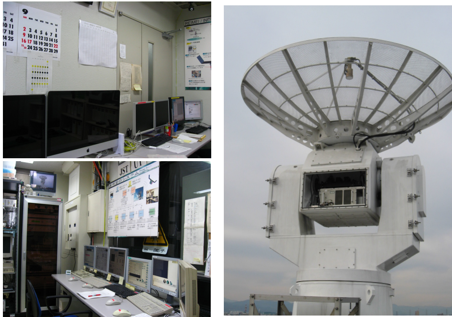
Figure 2.3: (Left) A look inside Reimei operation room. Several PCs for sending a variety of commands and displaying satellite status are put into the room. (Right) Communication antenna with diameter of 3 m installed on the roof of ISAS building at Sagami-hara .
